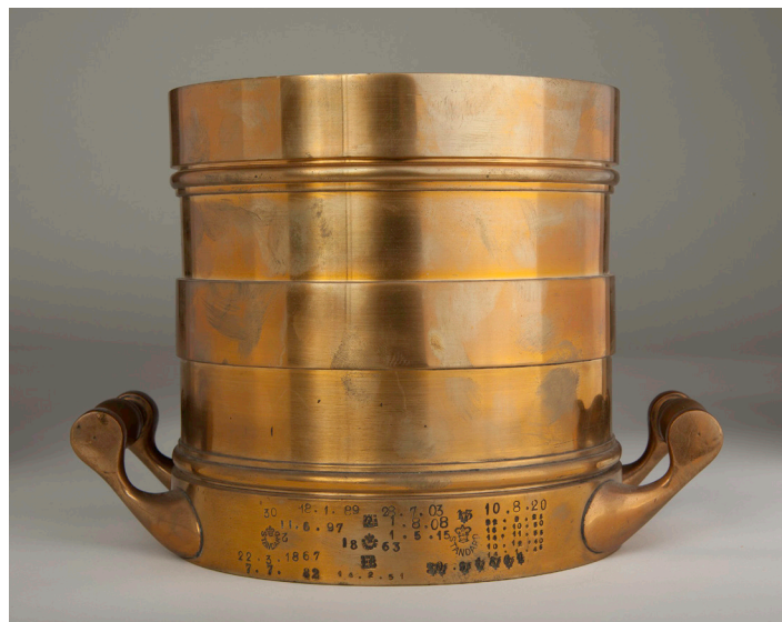
Figure 3: Item ST 42808 from Museums Victoria Collections, standard volume, imperial half gallon, primary standard, brass, potter, England, 1863.[7]
